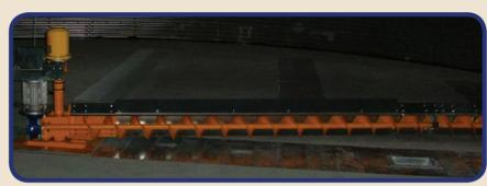
Sweep augers rotate around the centre point of the silo. The augers allow for the product to be completely emptied from the silo to save time and stock.
